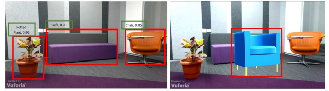
Figure 5: Bounding boxes for all the objects with labels and confidence score from the camera frame (left). Bounding box for the virtual chair (3D model) from the screenshot frame (right).
